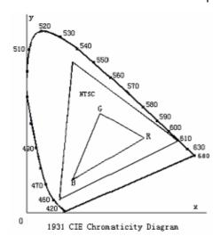
$$S = \frac{area \text{ of } RGB \text{ triangle}}{area \text{ of } NTSC \text{ triangle}} \times 100\%$$
