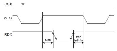
Note: Logic high and low levels are specified as 30% and 70% of VDDI for Input signals.
