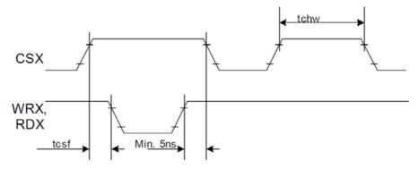
Note: Logic high and low levels are specified as 30% and 70% of VDDI for Input signals. Write to read or read to write timings:
