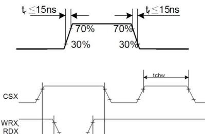
Note: Logic high and low levels are specified as 30% and 70% of VDDI for Input signals. Write to read or read to write timings:
